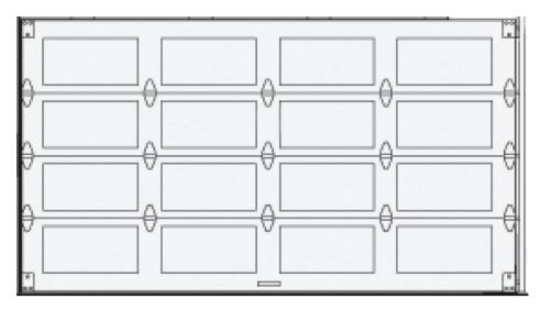
Total Door Area 20m<sup>2</sup> - single dwelling, max door weight up to 286kg when beams are installed
