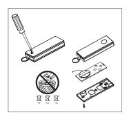
To replace battery for E945M & optional remote control transmitters - E943M & E940M, use a screwdriver blade to pry open the case as shown. Insert battery positive side up.
