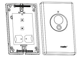
NOTE: The wall control supplied with your opener should be pre-programmed by the factory. If adding a new wall control, program into the opener before mounting the unit as detailed in section 18.
