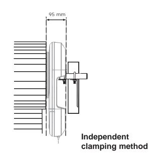
Ensure that there is at least 45 mm from the edge of the curtain to the edge of the bracket. If the roller door drum is on the edge of the curtain or is a smaller diameter, additional clearance may be required.
